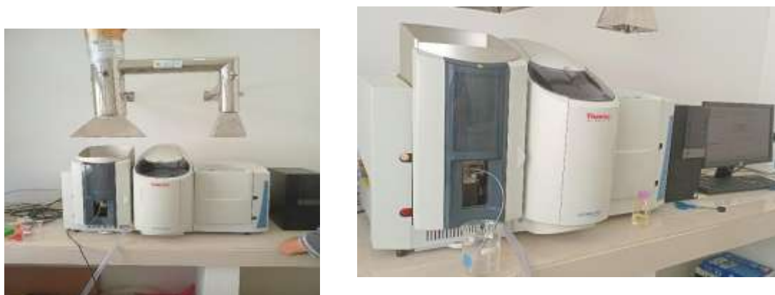
Gambar 2. 4. Atomic Absorption Spectrophotometer (AAS) Thermo Scientific Model iCE 3000 Series di Laboratorium Analisis Instrumentasi dan Penelitian Departemen Kimia.
