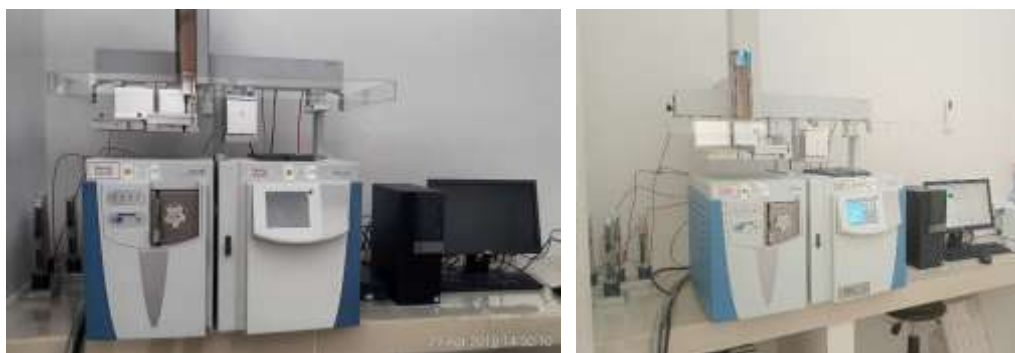
Gambar 2. 3. Gas Chromatography–Mass Spectrometry (GC-MS) Thermo Scientific model ISQ 7000 di Laboratorium Analisis Instrumentasi dan Penelitian Departemen Kimia.
